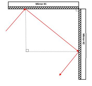
3. The picture to the right (which opens the video) shows a pair of mirrors. Note that the angle between the mirrors is slightly less than 90°. When a marker is placed before the mirrors, note that 4 images of the marker are seen by a centrally located observer.
